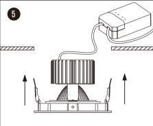
Clip upward and place the product in the hole in the ceiling.
