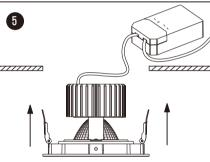
Clip upward and place the product in the hole in the ceiling.
