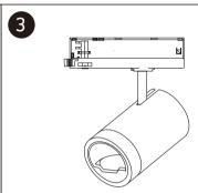
Rotate adaptor lock B clockwise to connect the adaptor to the neutral circuit.
